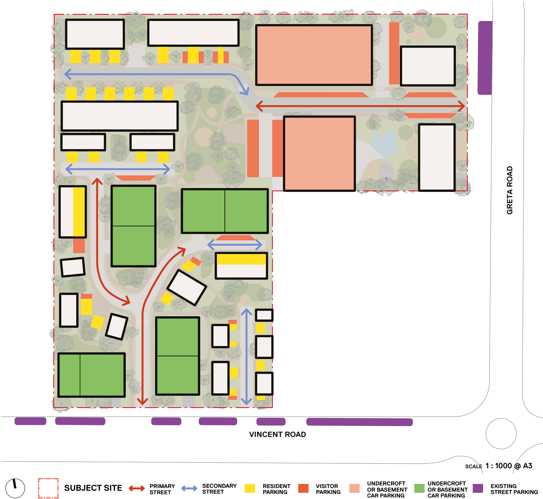
Figure 12: Access & Car Parking Locations
