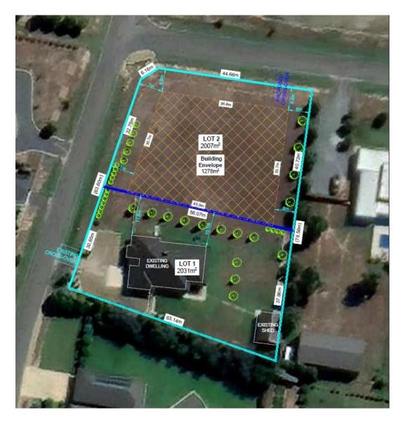
The southern-most lot, proposed Lot 1, would be generally rectangular in shape and have an area of  $2,031m^2$  with a 30m frontage to Pin Oak Drive. Access to the lot would be via the existing crossover on Pin Oak Drive. The existing dwelling and an associated outbuilding would be contained within proposed lot 1.
